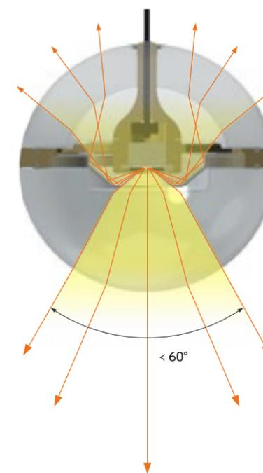
The core houses the LED, heat sink and holographic filter, which is responsible for producing a more uniform light. The core is accessible for maintenance by simply unscrewing the lower hemisphere.
