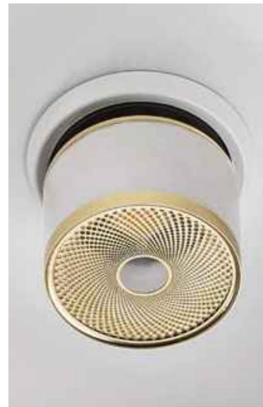
The lower filter made of photo-etched brass foil enables glare reduction and optimal light distribution. The dissipation system, developed and produced inhouse, guarantees the correct operating temperature of the LED. Both the heat sink and the central structure of the lamp are made of turned aluminium using the latest technologies of numerical control (CNC) machines.
