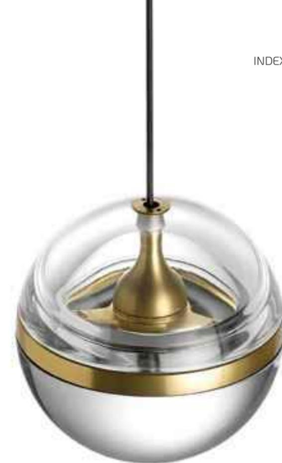
The upper hemisphere is designed to protect internal components and the silicone seals make the lamp body impervious to external agents. The 3-spoke aluminium center ring is made in-house using state-of-the-art computer numerical control (CNC) lathes. It is the key structural element of Limbus, as it supports and connects all the components of the lamp. At the center of the sphere, the crown-shaped element perfectly directs light and illuminates Limbus' crystal body.
