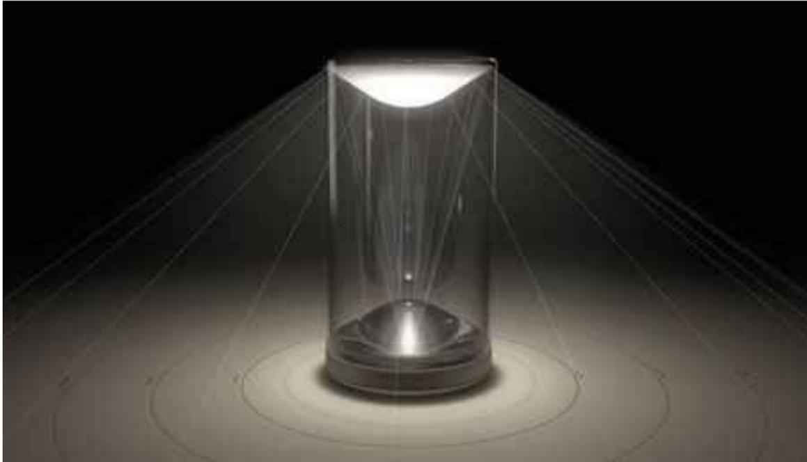
In Eve and Eva, the light flux is projected through a holographic filter, a small primary lens and a large secondary lens on the upper opaline cone, while the LED source remains hidden. Both lamps also have a tactile dimension: while with Eve the light is dimmed by a touch dimmer, with Eva it is dimmed by a rotary dimmer, which, thanks to an encoder system (an infrared sensor to detect rotation), allows the light intensity to be precisely controlled by manually actuating the ring on its base.
