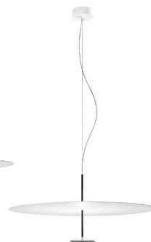
Dot consists of two parallel discs of different sizes, connected by a thin metal tube. The smaller, lower body is made of turned aluminium and contains a ring of LEDs optically designed to project a large amount of light onto the upper, lacquered aluminium reflector disc.
