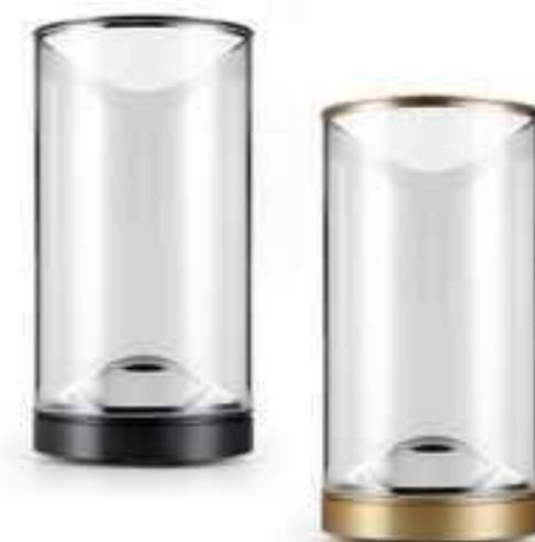
A natural development of Eve, Eve is a floor lamp similar to its big sister, but smaller in size and with a reduced light emission. Eve is a lamp with indirect light: the light source housed in the base emits a beam of light upwards, which passes through a PMMA lens, pointing at the upper conical reflector that acts as a diffuser. Dual-intensity touch dimmer on the base.
