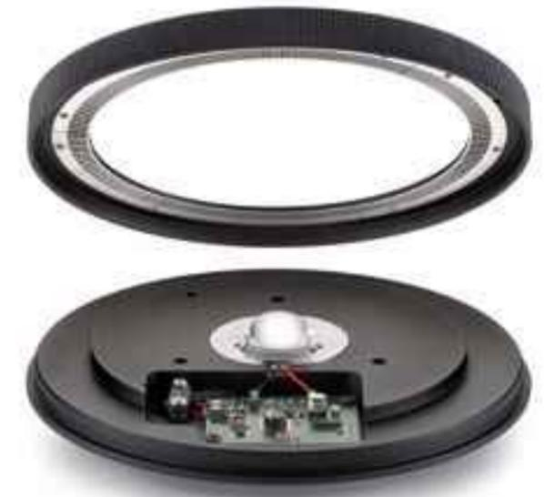
Rotary dimmer mounted on Eva's base with infrared sensor to detect rotation and adjust light intensity.
